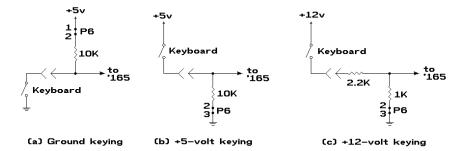
The resistor values shown are for 74HC ICs. If using 74LS, change the 10K resistors in (b) to 1K.
