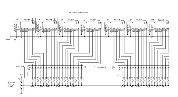
The 64 keys connect via two 34-conductor ribbon cables to connectors P4 and P5, 32 to each cable. The 64 resistors can be connected to either ground or +5 volts via a Keyboard Polarity Select jumper at P6 - if the keys go to ground, then the resistors go to +5 volts Vcc, and vice versa. A two-instruction change in the program in the microcomputer can accommodate either polarity, but I am using resistors to +5 volts and switches to ground.
