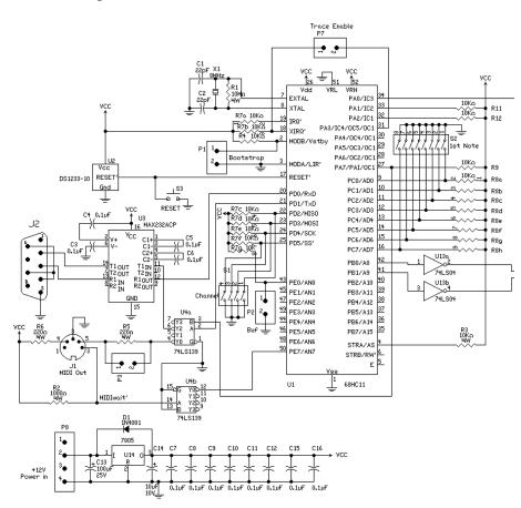
(a) Top left is the 8 MHz crystal and attached circuitry, which sets the speed of the processor. The 68HC11 internally divides this by 4, so the main clock frequency of the processor is 2 MHz.
