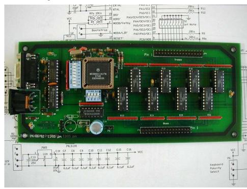
The drawings above show the revision B PC board, whereas the photograph is of a slightly earlier revision A board which worked fine, but lacked reset switch S3.
