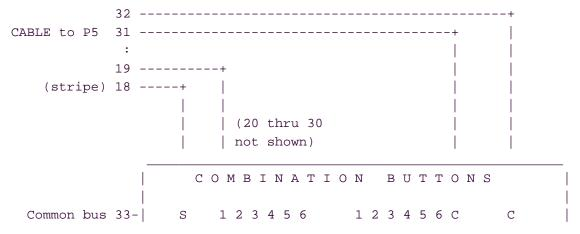
The pin numbers shown above are the pins on the MD-1 card's connector P4. In reality, the cable has only 17 wires, and pin 18 on the connector is the red-striped wire on the cable (which would normally be called pin 1). Hence
