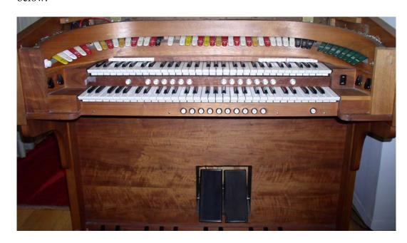
These buttons are wired to the same MD-1 as the pedals. An MD-1 has 64 inputs in the form of two 34-pin ribbon connectors. But organs have a maximum of 32 pedals (and my theatre organ only has 25). Thus one whole 34-pin connector (and a few pins on the other) are totally unused. This cable uses this second 34-pin connector (P4) to process inputs from these extra combination buttons. There are still unused inputs left over, and these may be used in the future for other applications.
