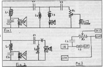
HF-1. The X marks the place where the connection is severed when an HF-1 is installed. Figure 3 is a schematic of the "mystery" box.
